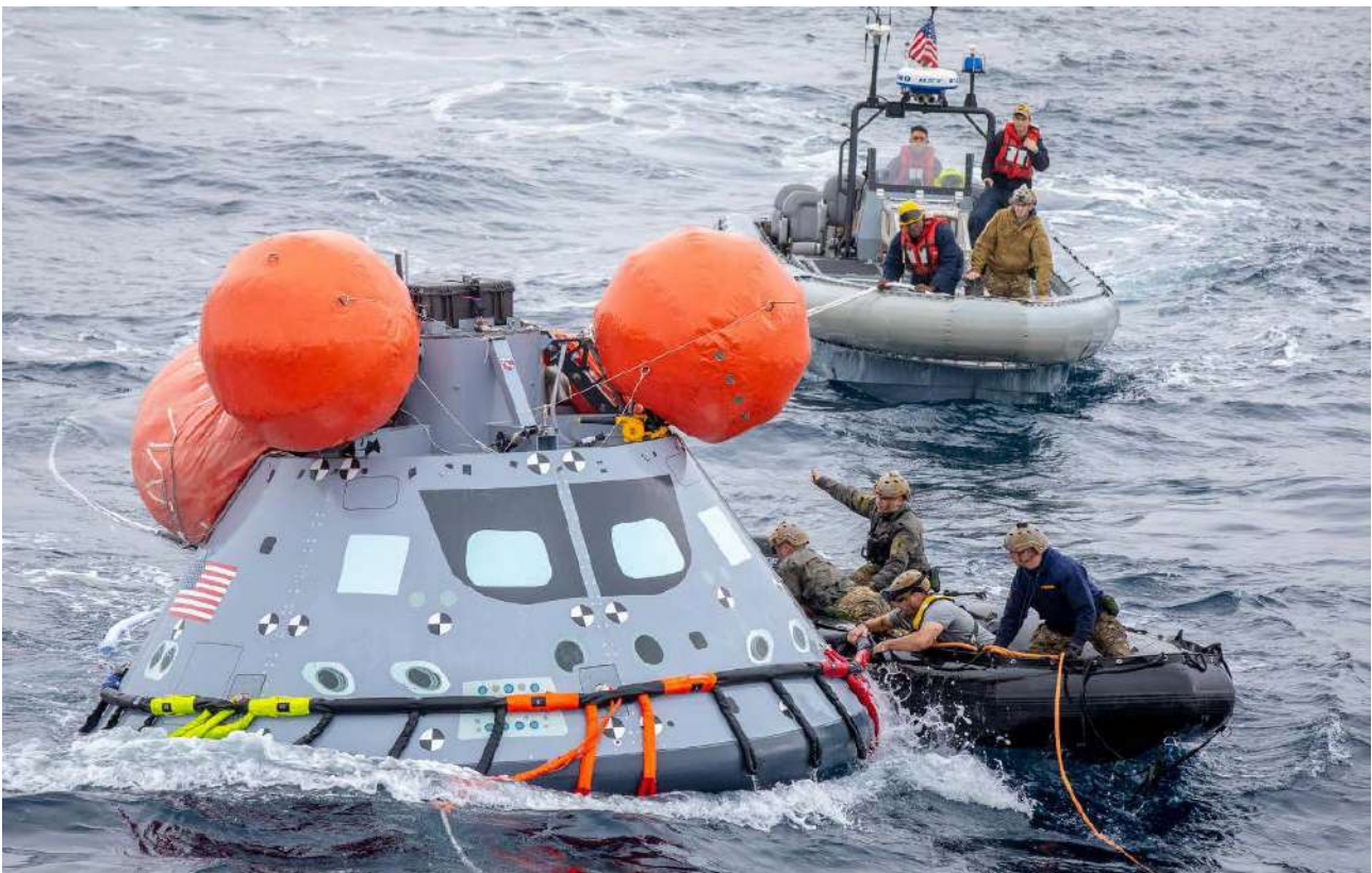
U.S. Navy divers from Explosive Ordnance Disposal (EOD) Expeditionary Support Unit 1, attach tending lines to a mock Orion capsule during Day 2 of Underway Recovery Test 9 (URT-9) aboard the USS John P. Murtha. During the weeklong test, NASA's Landing and Recovery team completed their final mission certification ahead of Artemis I.
