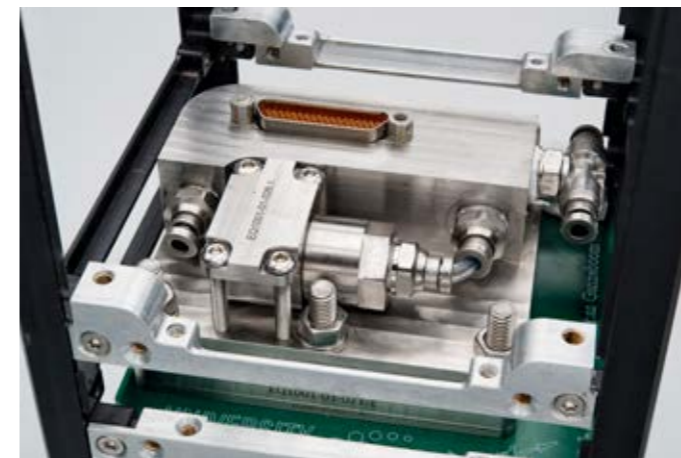
Detail of the multi-parallel micro-pump
